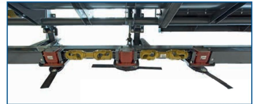
The Independent Row Unit Head can be equipped with a Stalk Chopper Kit. The cutting system is composed of blade discs with mechanical gearboxes and it covers the entire harvesting length. A cardan shaft activates the system mechanically from the right side of the transmission channel of the combine. The adjustment of the cutting height is hydraulically driven from the combine cab.
